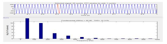
Fig.8.total harmonic distractions for 17 Level inverter.
