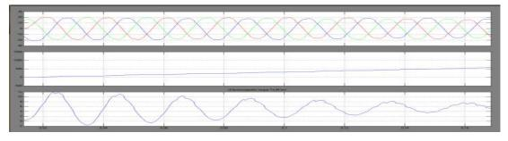
Fig 15. Three Phase voltage and three phase IM voltage, speed and torque for 25-level inverter
