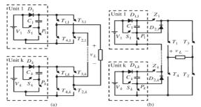
Fig.2. (A) First Proposed Topology. (B) Second Proposed Topology.
